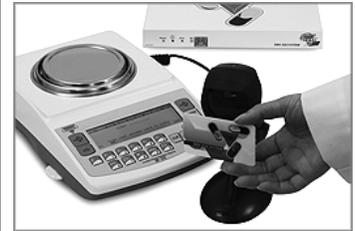
1. Place a vial or a counting container on the pan and press the “T” key to tare.
