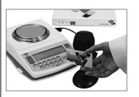
1. Place a vial or a counting container on the pan and press the "T" key to tare.
