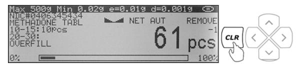
**Note:** A count down meter in the upright corner of the display indicates the progress of the count. A count of 0 means the script is filled. If too many pills are placed into the container the "Overfill" indicator will be displayed.
