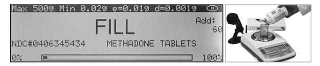
7. Stop filling when the count has been reached and press the "CLR" key to complete the transaction.
