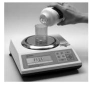
**Note:** If filling does not begin while the command "Fill" is displayed, after approximately 5 seconds the scale will display 0 pcs
