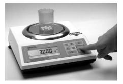
Note: Minimum individual piece weight allowed is 30mg (3e). With a sample size of 10 pieces, the sample weight must be equal to or greater than 300mg (30e). Attempting to set a sample size of 10 pieces with a total sample weight which is lower than 300mg (30e) will result in a Sample Low error (SAPL-LO)
