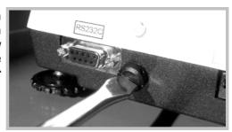
Once the wire seal screw has been removed and the calibration switch exposed, gently insert the flush sealing screw provided with the scale in the place of the wire seal screw.
