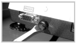
2. Once the screw has been removed and the calibration switch exposed, use a pen or another pointing device to toggle the calibration switch to the right (which is the ON position.)
