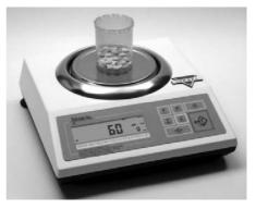
14. Once an accurate piece count has been taken, the container and its contents may be removed from the scale. After removal of the container with the counted pieces, the scale will indicate the count is finished and that a new count may be initialized by pressing the "C" key. The command "----, COUNT FINISH, TO START COUNT PRESS C" will appear on the display sequentially.
