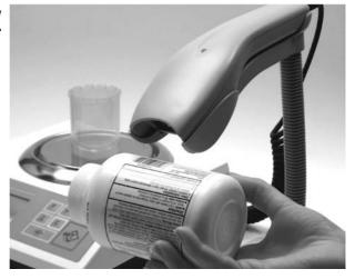
7. The scale will then ask to select a sample size. Because the minimum sample size is 10 pieces, the scale automatically selects "SPL-10" which is sample size 10. The sample may be changed either to 30 pieces or 60 pieces by pressing the sum button ( $\Sigma$ ).
