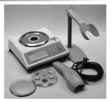
2. After removing the pan base and the pan from their packaging, carefully install the pan base onto the scale by placing it on the pan support located in the middle of the scale. Once the pan base has been installed, carefully place the pan on the base as shown below.
