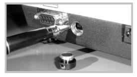
3. Upon toggling of the calibration switch, the balance will go into Calibration Mode. For approximately five (5) seconds the display will read CAL, indicating the scale is in Calibration Mode.
