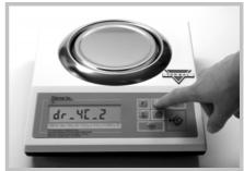
2. The scale will then display commands Set-t-O, and Set-t-1 appearing sequentially approximately every 2 seconds. To change the date and time, press the "T" key while command Set-t-1 is displayed. If you want to cancel the operation, press the Tkey while Set-t-O is displayed.
