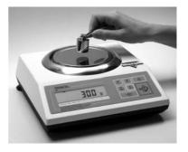
7. When the 300g weight is placed on the pan, the scale will automatically begin the calibration process. The display will read "C" which means the scale is calibrating. Because calibration is a very sensitive process, make sure the scale is not exposed to any air movements or vibrations.
