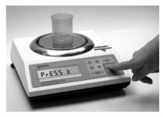
5. Once the scale has finished taring, "Scan" will appear on the display indicating you should scan the NDC code associated with the drug.
