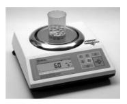
9. Once an accurate piece count has been taken, the container and its contents may be removed from the scale. After removal of the container with the counted pieces, the scale will indicate the count is finished and that a new count may be initialized by pressing the "C" key. The command "----, COUNT FINISH, TO START COUNT PRESS C" will appear on the display sequentially.
